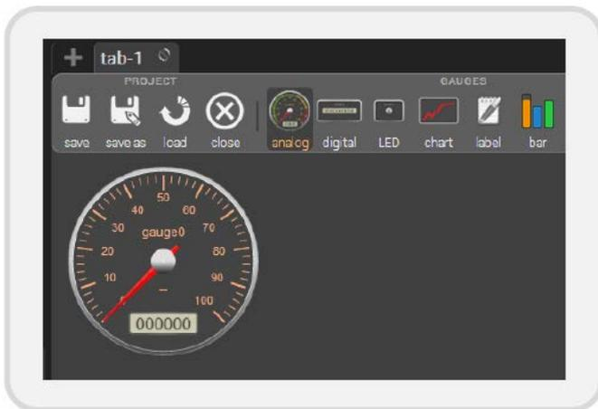
Each gauge has specific parameters that can be configured that are unique to each gauge. The common thing throughout most gauges is the signal field. That is where the reference between a gauge and a specific variable from the data modules can be established so the gauge can display the data contained by the referenced variable.
